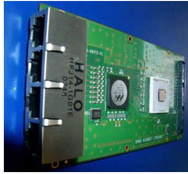
Figure 5.5: Quad copper Gigabit Ethernet mezzanine card (photo taken from [47]).
