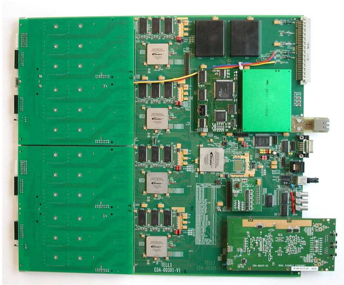
Figure 5.35: TELL1 prototype with mezzanine cards mounted.
