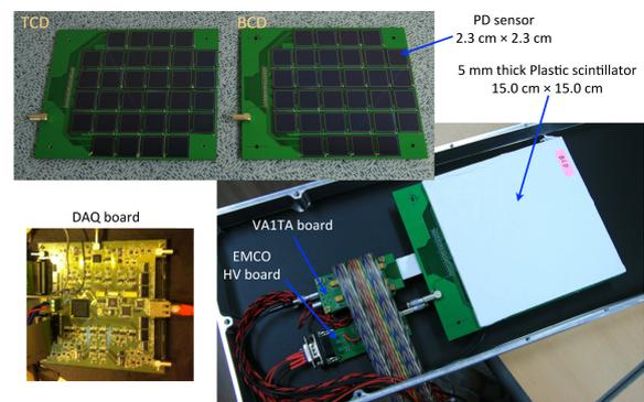
Fig. 8: Prototype TCD/BCD for the CERN beam test.
