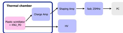
Fig. 4: Detector cell components used for the thermal test.
