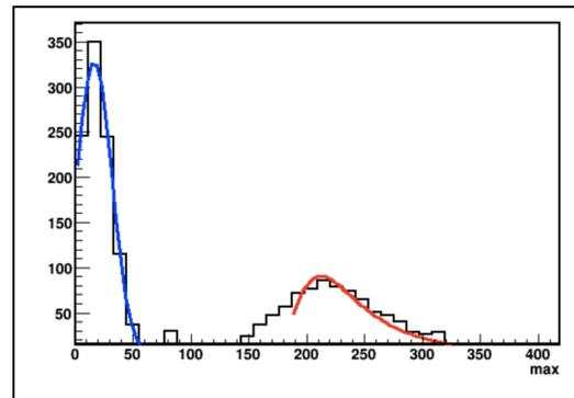
Fig. 3: Signal-to-noise ratio distribution obtained with the  $^{90}\text{Sr}$  radioactive source.
