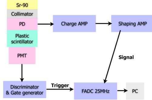
Fig. 2: Block diagram of the SNR measurement system.
