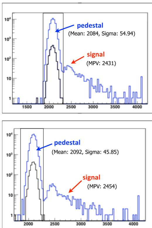
**Fig. 9:** Pulse-height distribution of two channels on the prototype BCD at the CERN beam test.
