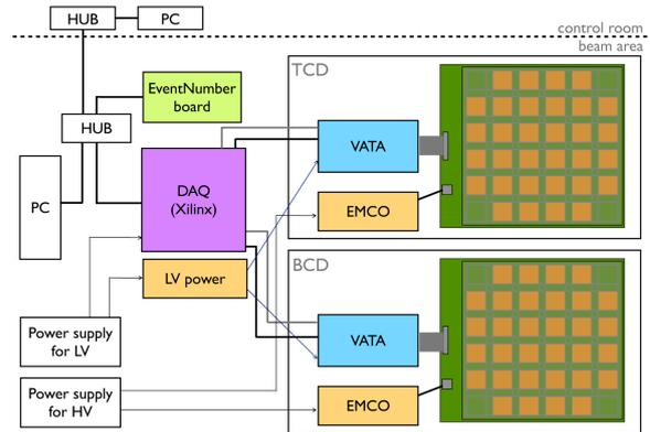
Fig. 7: Block diagram of the CERN beam test system.
