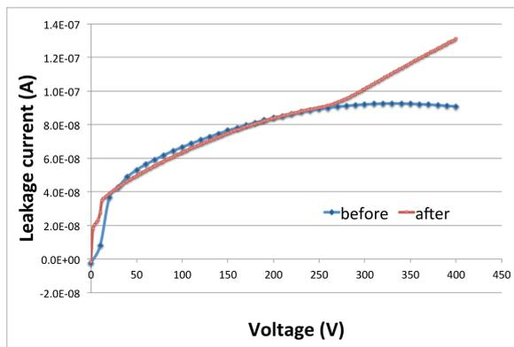
Fig. 6: I-V curve of the detector cell component before/after vacuum test.
