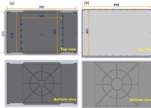
Fig. 1: Schematics of the (a) TCD and (b) BCD enclosures.
