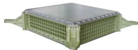
Fig. 2: The honeycomb structure of the electromagnetic calorimeter of the AMS-02 detector
