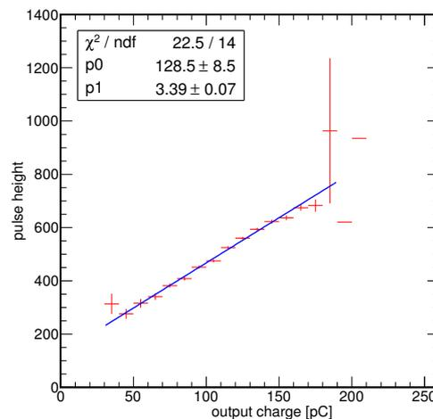
**Fig. 7:** The beam charge dependence of the observed signals. The horizontal axis is the output beam charge measured at the ELS. The vertical axis is the pulse height of the observed signal at the receiver.
