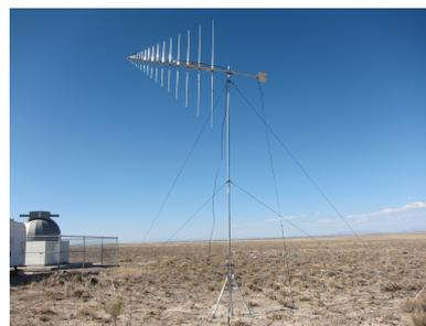
**Fig. 3:** Installed log-periodic antenna in TA site.
