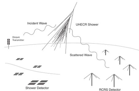
**Fig. 1:** The geometry for a radar echo technique.
