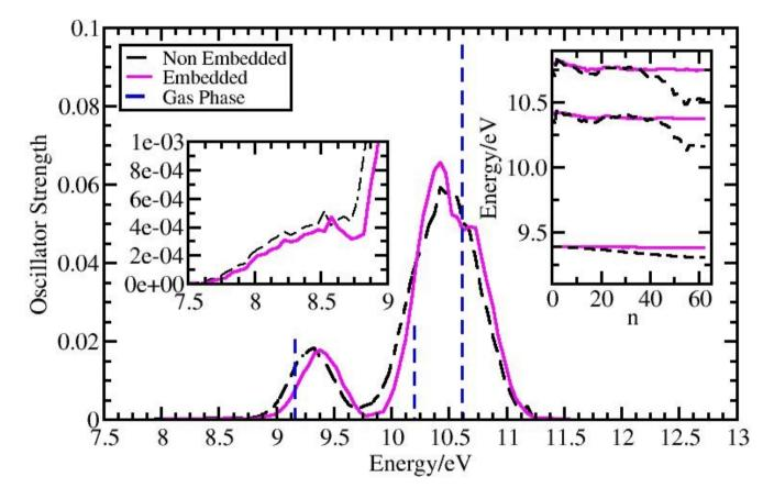
The peak position of the first absorption band (L) is blue-shifted by 0.2 eV relative to the gas-phase value.
