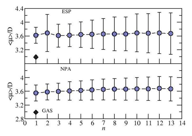
Significant change on the average monomeric dipole moment of HCN from 2.9 (G) to 3.6 D (L).
