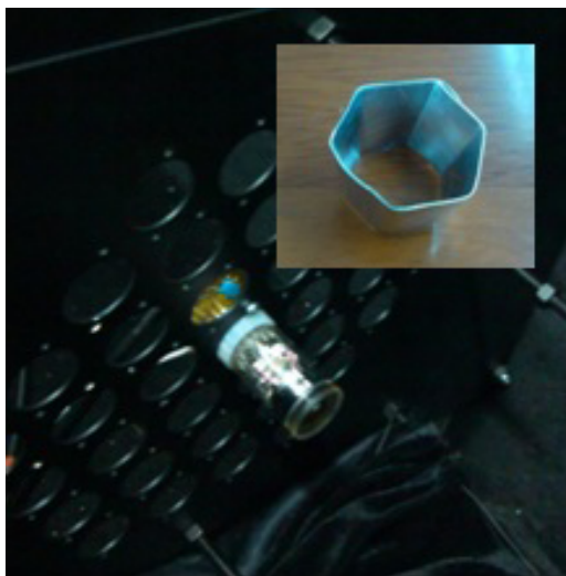
Fig. 6: The photomultiplier black-box testing system and insertion is a simple light cone made of aluminum foil.
